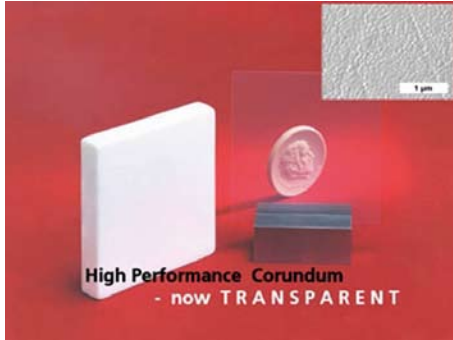
Transparent aluminium-oxide ceramics based on nanoparticles (IKTS)
