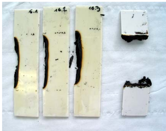
Fig. 2: ABS samples (thickness 3 mm) after horizontal burning test. Left modified with flame resistant coating (0.1 mm), right pure ABS control.
